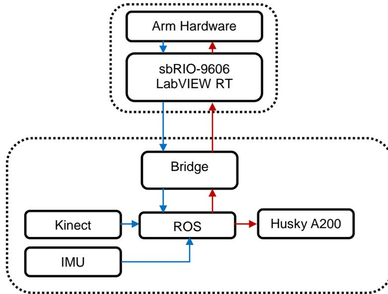
Figure 10: Architecture of a Mobile Manipulator
