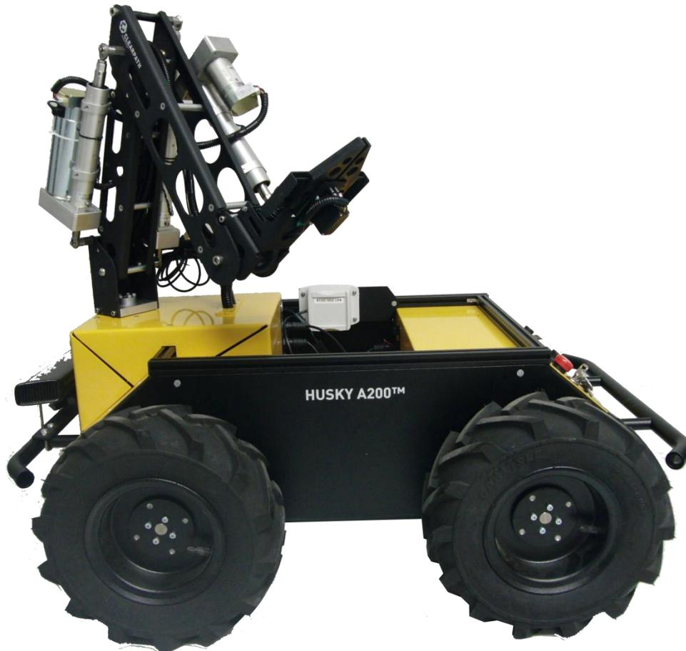
*Figure 9: Husky A200 equipped with custom manipulator*
