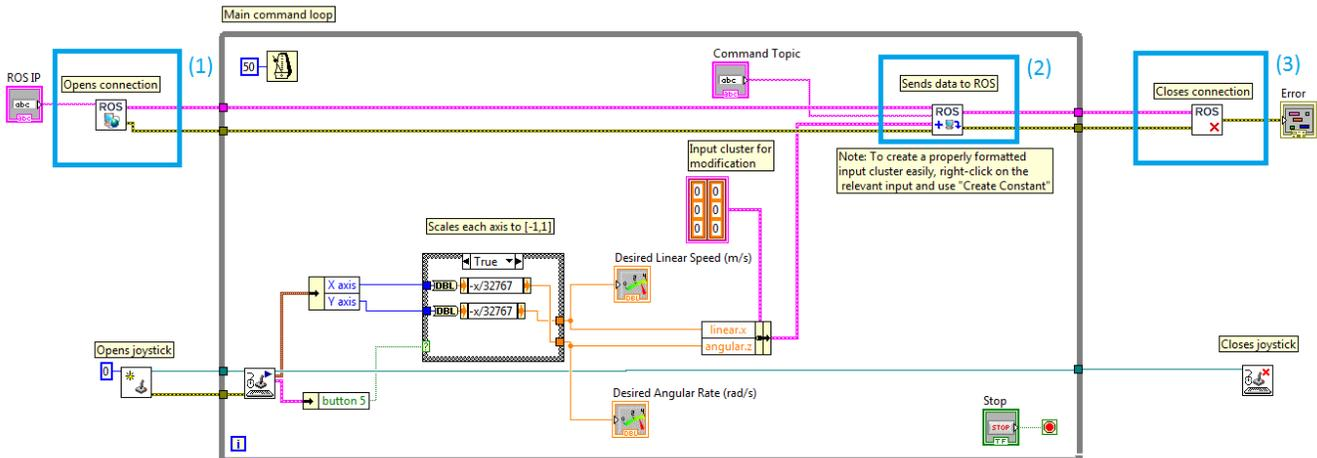
Figure 3: Using ROS Toolkit to control a mobile robot
